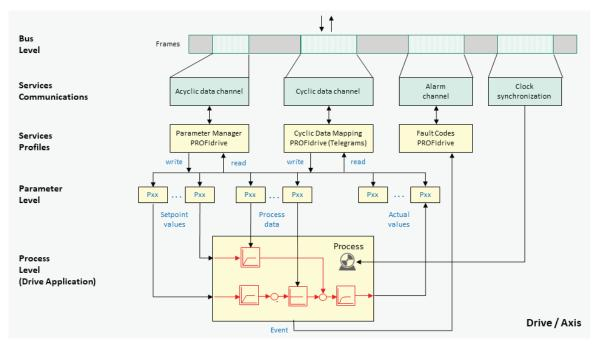
Fig. 4: Data model and data flows in a drive axis or PROFIdrive drive object (DO)
