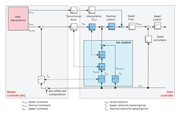
Fig. 12: Dynamic servo control (DSC) concept
