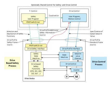
Fig. 15: Integration of drive-based safety in the drive device
