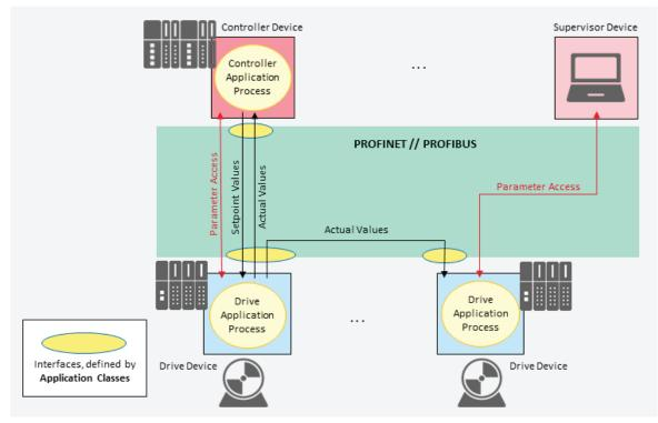
Fig. 2: General PROFIdrive drive application model
