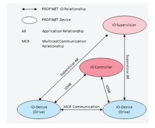
Fig. 18: Mapping of base model to PROFINET IO
