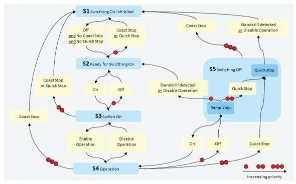
Fig. 6: Basic state machine of a PROFIdrive drive axis
