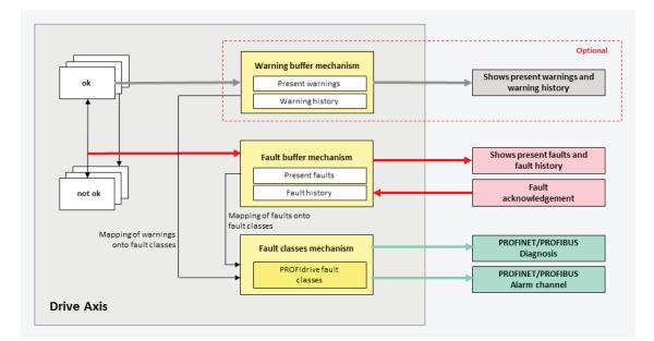
Fig. 14: PROFIdrive diagnostic functions
